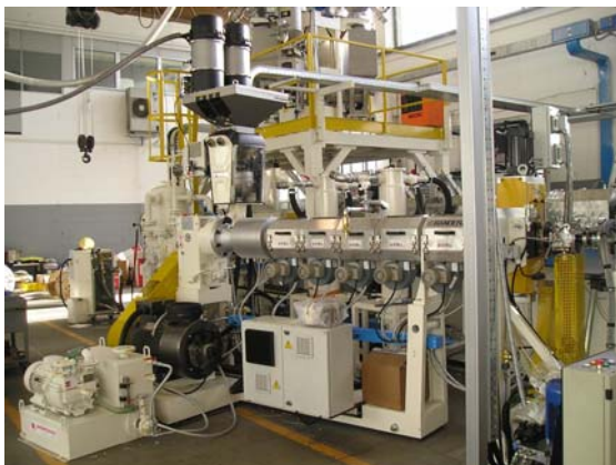
SINGLE SCREW CO-EXTRUDER 35:1 L/D WITH NEW VACUUM VENTING SYSTEM TO AVOID VIRGIN PET DEHUMIDIFICATION FOR EXTERNAL SKIN LAYERS
