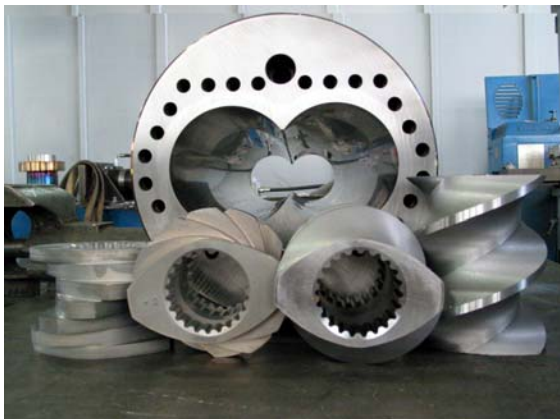
SCREW AND BARREL COMPONENTS OF TWIN SCREW CO-ROTATING EXTRUDER
