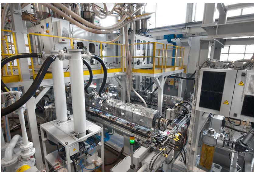
BETA PET LINE: EXTRUSION SECTION AND LINE PC SUPERVISOR (17" TOUCH SCREEN)
