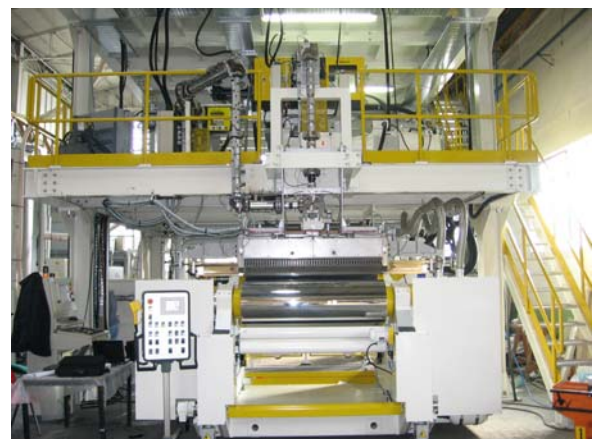
PARTICULAR-DESIGNED “TAILOR MADE” MULTILAYER PET FOIL EXTRUSION LINE
