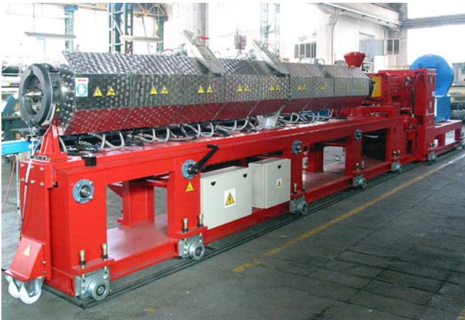
TWIN SCREW CO-ROTATING EXTRUDER MOD. 2C 105mm – THROUGHPUT PROCESSING PET FOIL: 1300Kg/h
