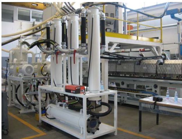
SCHEME AND PHOTO OF THE NEW TWIN SCREW CO-ROTATING EXTRUDER VENTING DEGASSING SYSTEM
