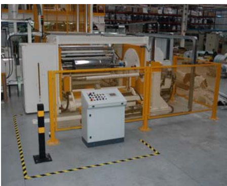
FULLY AUTOMATIC WINDING SYSTEM FOR MULTI-REEL PRODUCTION: TURRET-REVOLVER, CANTILEVER OR TROLLEY
