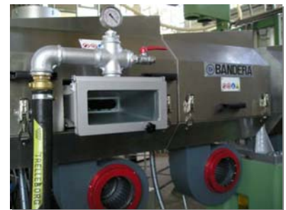
SOME PARTICULARS OF SINGLE SCREW EXTRUSION SYSTEM EQUIPPED WITH VENTING DEGASSING DEVICE
