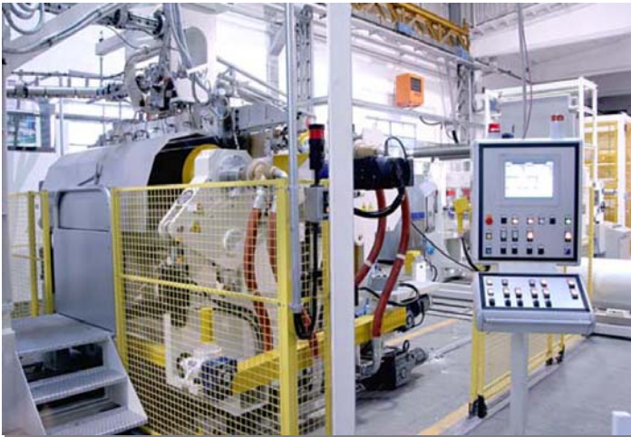
CALENDER ROLL STACK SECTION
