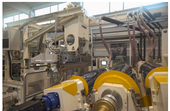
ONE OF THE MOST RECENT BANDERA PET FOIL EXTRUSION LINE SUPPLIED – YEAR 2010
