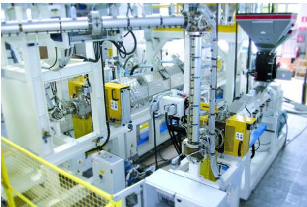
ALFA PET LINE: EXTRUSION SECTION AND ROLL STACK CALENDER GROUP
