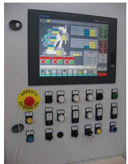
BETA PET LINE: EXTRUSION SECTION AND LINE PC SUPERVISOR (17" TOUCH SCREEN)
