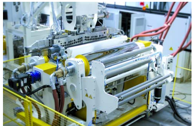
ALFA PET LINE: EXTRUSION SECTION AND ROLL STACK CALENDER GROUP
