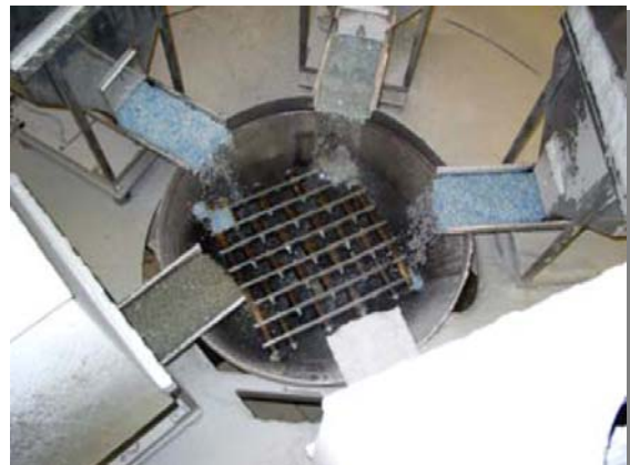
DOSING SYSTEM FOR BOTH VIRGIN AND REGROUND RAW MATERIALS
