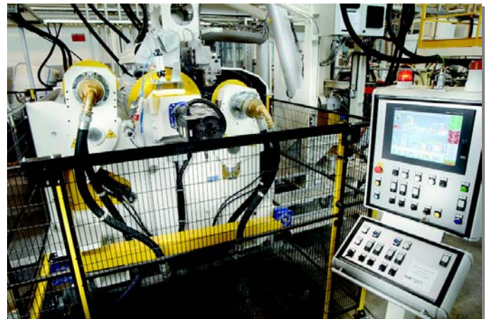
FROM PET BOTTLE FLAKES TO PET PACKAGE WITH BANDERA PET FOIL EXTRUSION LINE
