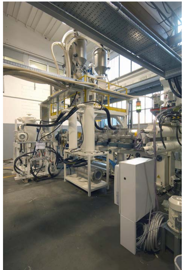
SCHEME AND PHOTO OF THE NEW TWIN SCREW CO-ROTATING EXTRUDER VENTING DEGASSING SYSTEM
