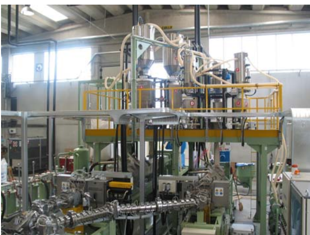
ONE OF THE FIRST BANDERA PET FOIL EXTRUSION LINE INSTALLED – YEAR 2000
