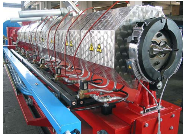
TWIN SCREW CO-ROTATING EXTRUDER MOD. 2C 105mm – THROUGHPUT PROCESSING PET FOIL: 1300Kg/h
