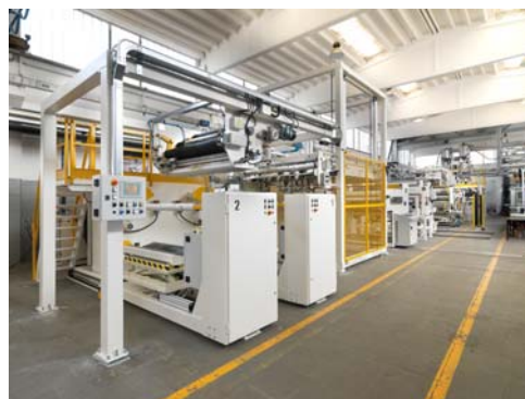
FULLY AUTOMATIC WINDING SYSTEM FOR MULTI-REEL PRODUCTION: TURRET-REVOLVER, CANTILEVER OR TROLLEY
