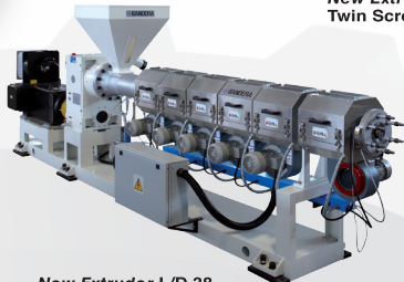
New Extruder L/D 38 Single Screw
